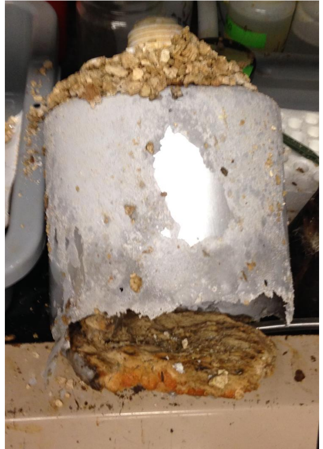
Two views of the actual container. The container itself actually failed thru the cap, the eating away of the container was done after the pressure had be equalized.
