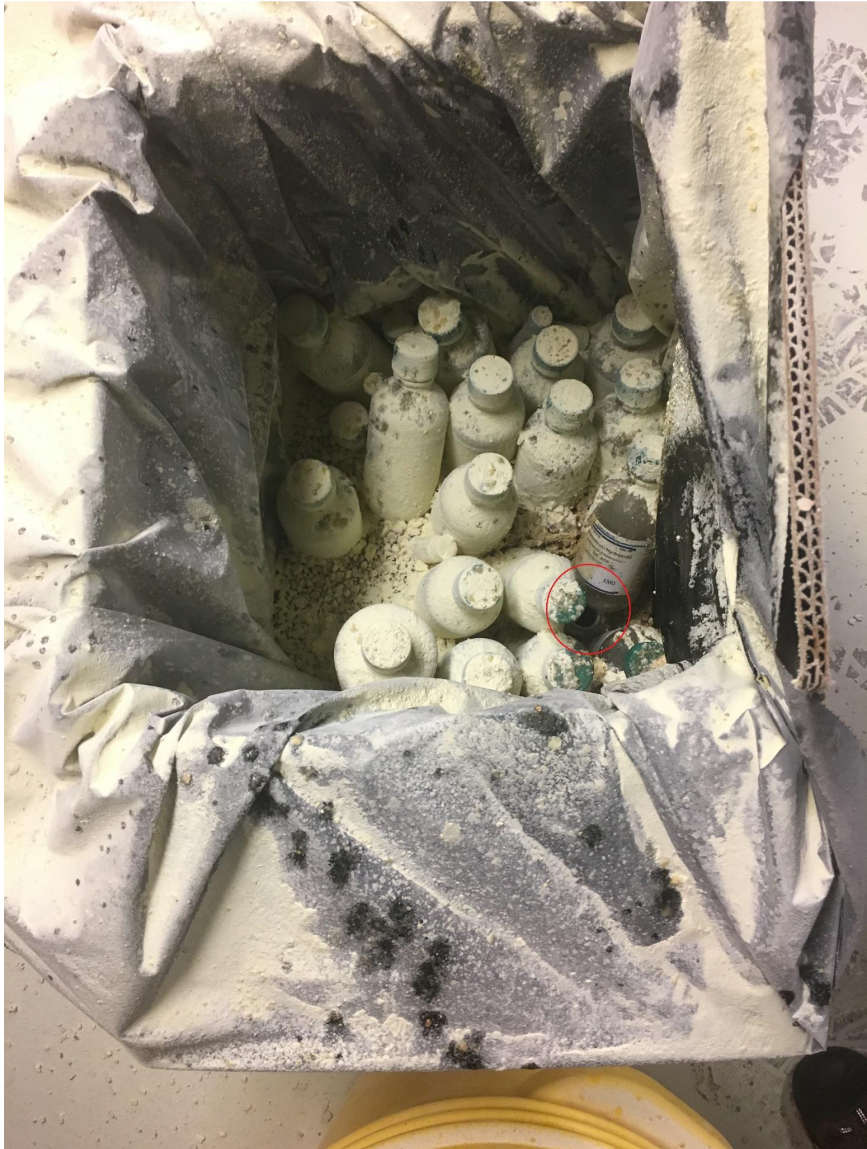
Looking inside the drum, the failed container is circled in red.
