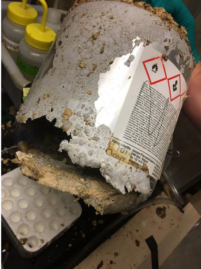
Two views of the actual container. The container itself actually failed thru the cap, the eating away of the container was done after the pressure had be equalized.
